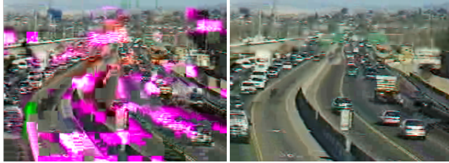
Fig. 4: Example of MPEG-4 decoding without PacketVideo error recovery and concealment (left) vs. PacketVideo error resilient decoding (right) in a 10^{-3} avg. BER W-CDMA channel.
